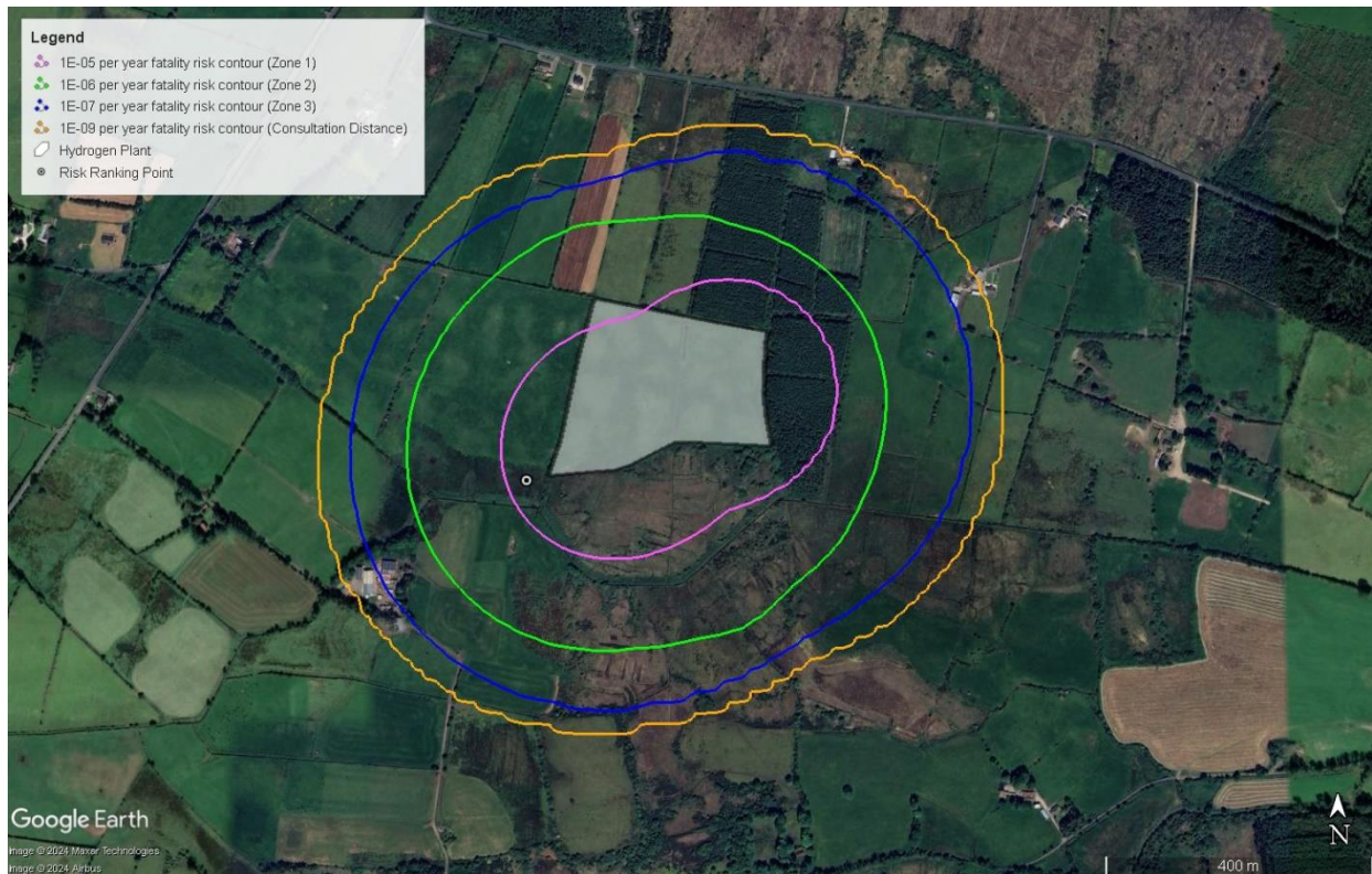
Figure 4-3: Risk Ranking Point – South-West – Inner Zone
